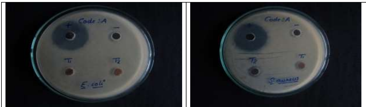
Fig.4a Antimicrobial activity against E.Coli and staphylococcus aureus for nickel nanoparticles using oxalic acid
